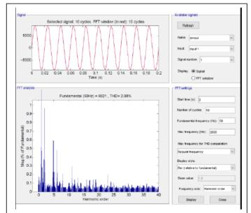
Fig.6. Harmonic analysis of phase A voltage sag caused by transformer energizing at 11 kV bus.
