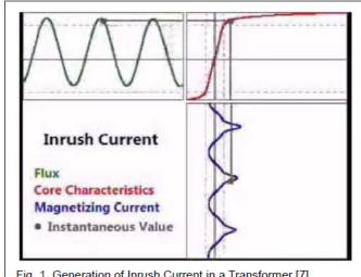
Fig. 1. Generation of Inrush Current in a Transformer [7].
